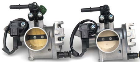
The primary modification performed by Injectioneering is the replacement of the throttle butterfly. The new one (on the right) sits at a different angle and has a compensation bleed hole.
