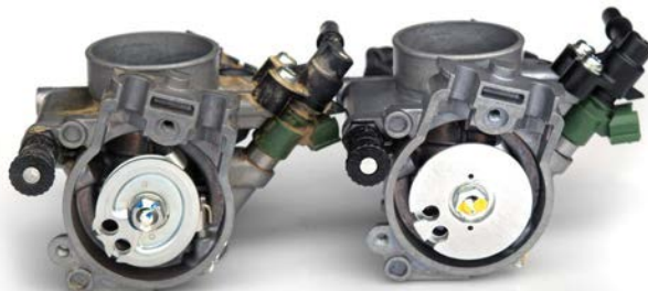
The YZ's stock throttle body pulley is oval-shaped, which results in the throttle opening at a faster rate initially. The round pulley makes the bike easier to manage.
